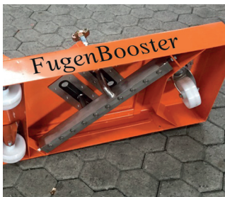
Integrated splash guard on the device
